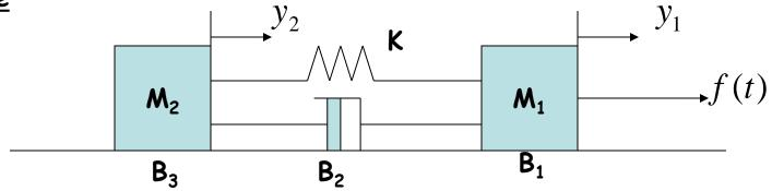
$M_1 \ddot{y}_1 + B_1 \dot{y}_1 + B_2 (\dot{y}_1 - \dot{y}_2) + K(y_1 - y_2) = f(t)$  $M_2 \ddot{y}_2 + B_3 \dot{y}_2 + B_2 (\dot{y}_2 - \dot{y}_1) + K(y_2 - y_1) = 0$
